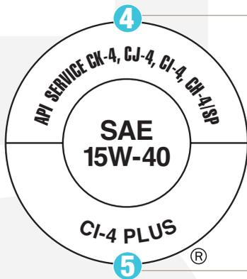
**2. Viscosity Grade** The measure of an oil's ability to flow at certain temperatures. Vehicle requirements may vary. Follow your vehicle manufacturer's recommendations on SAE oil viscosity.
