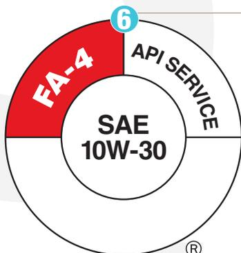
**3. Resource Conserving** "Resource Conserving" applies to oils intended for gasoline-engine cars, vans, and light trucks. Widespread use of "Resource Conserving" oils may result in an overall savings of fuel in the vehicle fleet as a whole.
