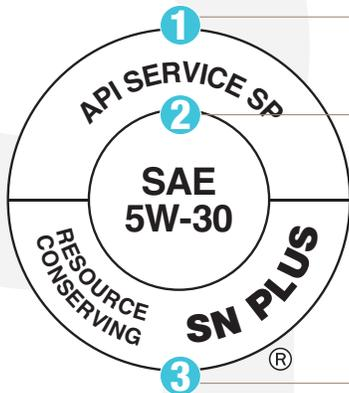
**1. Performance Level** Motor oils designed for cars, vans, and light trucks with gasoline engines fall under API's "S" (Service) categories. Motor oils designed for heavy-duty trucks and vehicles with diesel engines fall under API's "C" (Commercial) categories. Please see the Gasoline Engines and Diesel Engines charts on the next pages for descriptions of current and obsolete API service categories.
